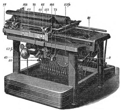
7-Ribbon-shifting, or Long-gear Shaft.
